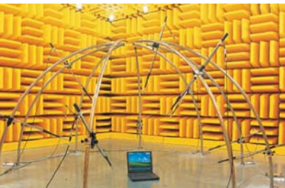
Anechoic Chamber for Noise Test
